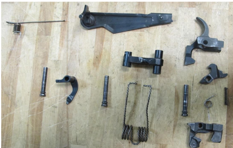
Figure 3: AKM type rifle components, including hammer and trigger mechanism springs (credit: N.R. Jenzen-Jones/ARES).
