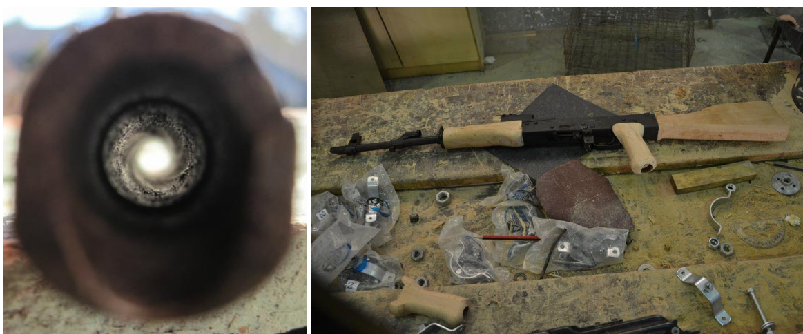
Figure 1: A badly corroded firearm barrel (credit: KIR).
