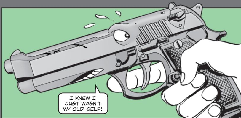
An M9 pistol that is fired frequently will develop cracks eventually. There's nothing you can do to stop cracks, but you can spot them before they crack up your M9.
